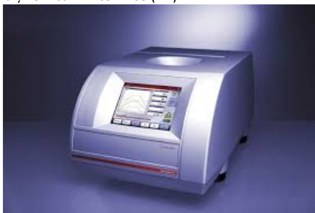
Figura 1. Reactor monomod Monowave 300 (Anton Paar, Graz, Austria)
